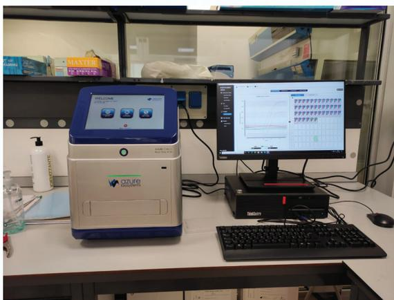
Azure Cielo Real-time PCR Biosystems
