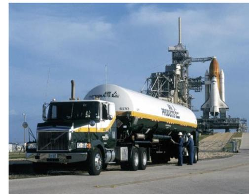
Liquid Hydrogen tank on truck
