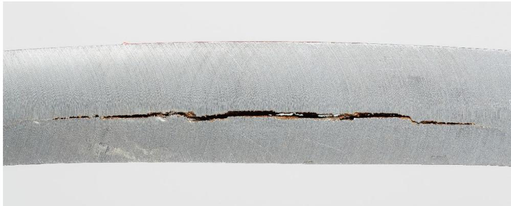
Hydrogen-Induced Cracks (HIC)
