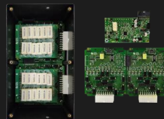
Battery Management System
